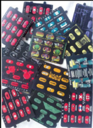
» [Jaguar] The keypad of the Jag's controller is major part of the gameplay experience and selected games came with special overlays to improve it further.
